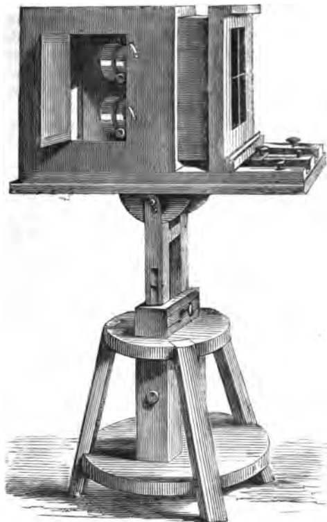
Fig. 46. Stand for Operating Room, and Camera for "Cartes de Visite."
